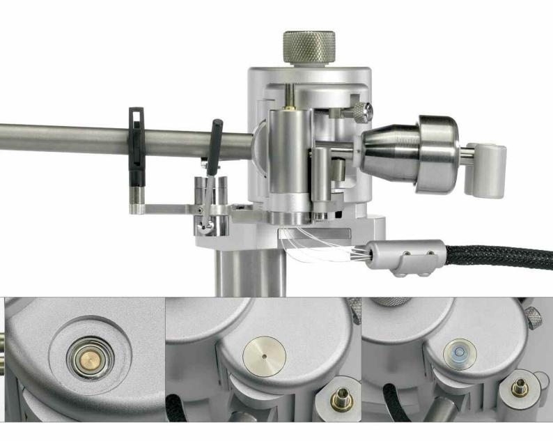
Above: It doesn't get better than this: The tonearm cable is made up of seasoned 5N pure silver wire, which itself consists of 36 individual Litz wires with a diameter of 3/100 mm constructed around a non-conductive core. The cable shows no restoring force thanks to the extremely thin single wires; it neither interferes with the rotary process, nor does it affect the skating forces. A cable such as this is almost unobtainable on the world market today
